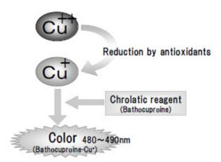
Samples are mixed with Cu++ Solution. Cu++ are reduced by antioxidants to form Cu+. Reduced Cu+ react with Chromatic Solution (Bathocuproine), and can be detected by absorbance at wavelength 480 to 490 nm. Antioxidant capacity can be calculated from the Cu+ formed.
